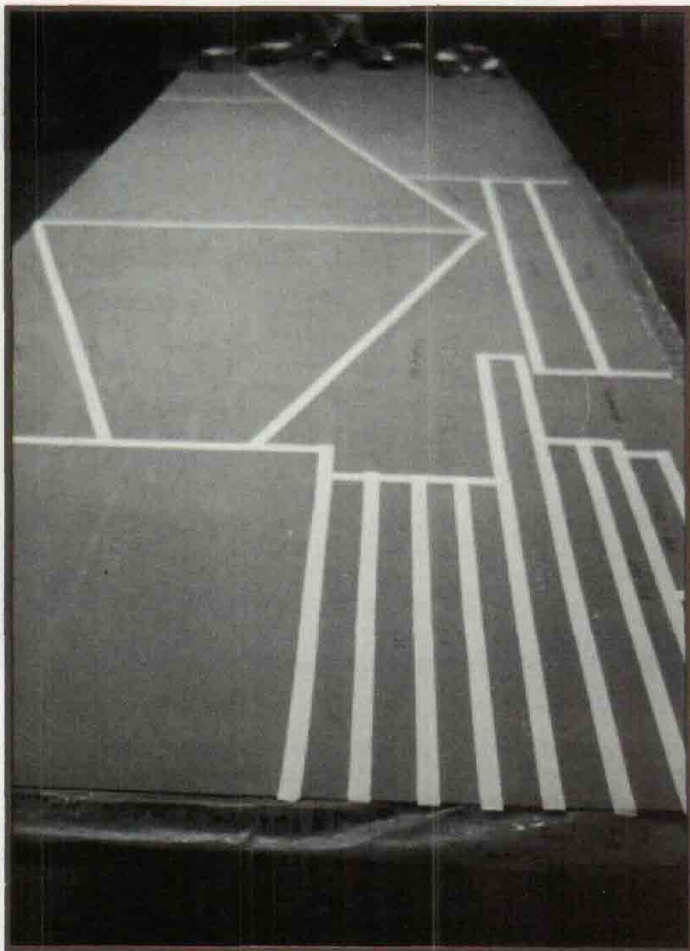
A sheet of aluminum skin for the author's Durand Mark V — cleaned, alodined, chromated, marked, taped and ready for cutting.
